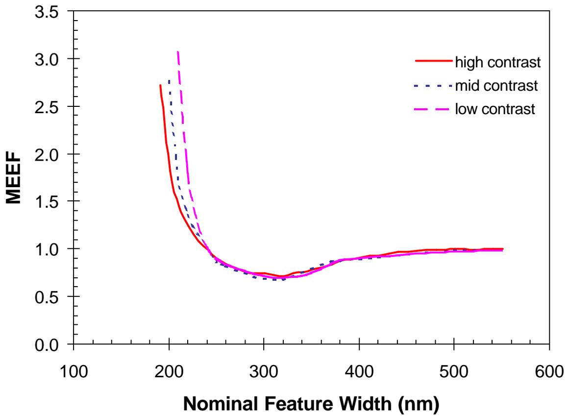
Figure 1. Resist contrast affects the mask error enhancement factor (MEEF) dramatically near the resolution limit.
