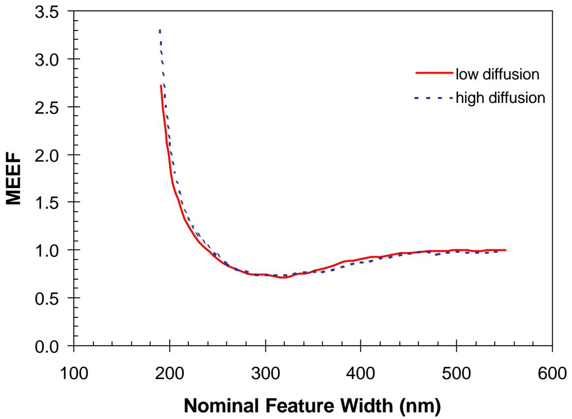
Figure 2. Increased resist diffusion has the same effect on MEEF as lower resist contrast.
