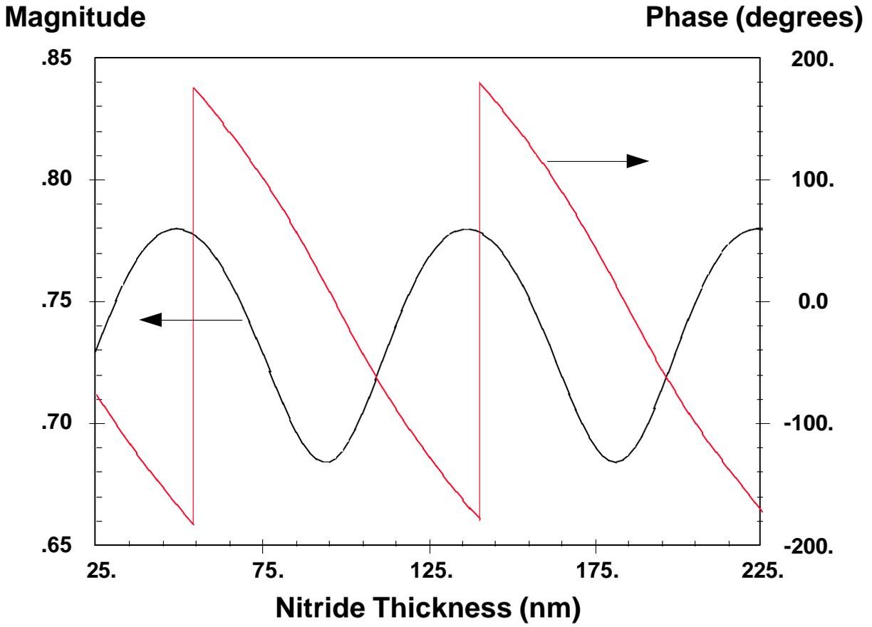
Figure 1. Variation of the magnitude and phase of the resist/substrate reflection coefficient as a function of silicon nitride thickness for a film stack of resist on nitride on 40nm of oxide on silicon.
