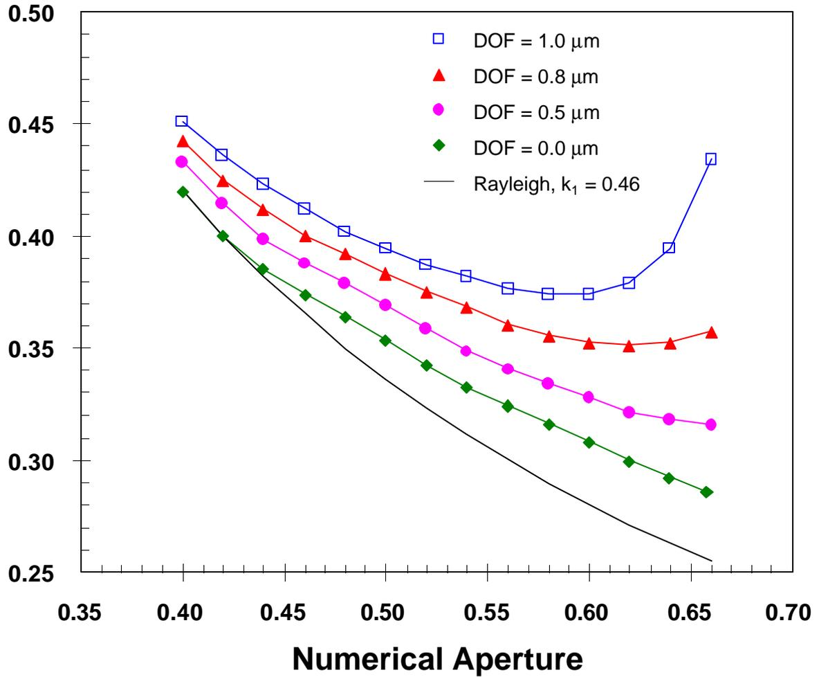
Figure 4. Resolution as a function of numerical aperture is more complicated than Rayleigh's criterion would imply.
