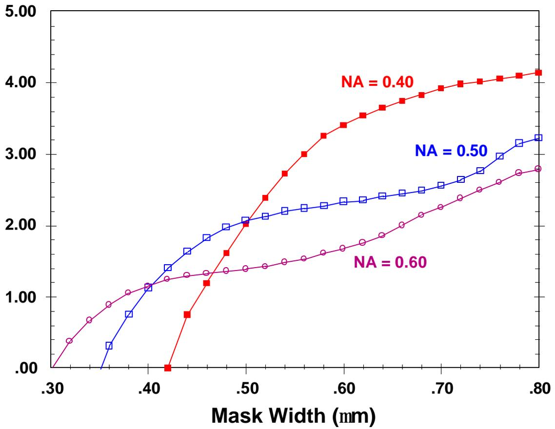
Figure 3. The definition of resolution can be used to study fundamental lithographic trends, such as the impact of numerical aperture (NA) on resolution.
