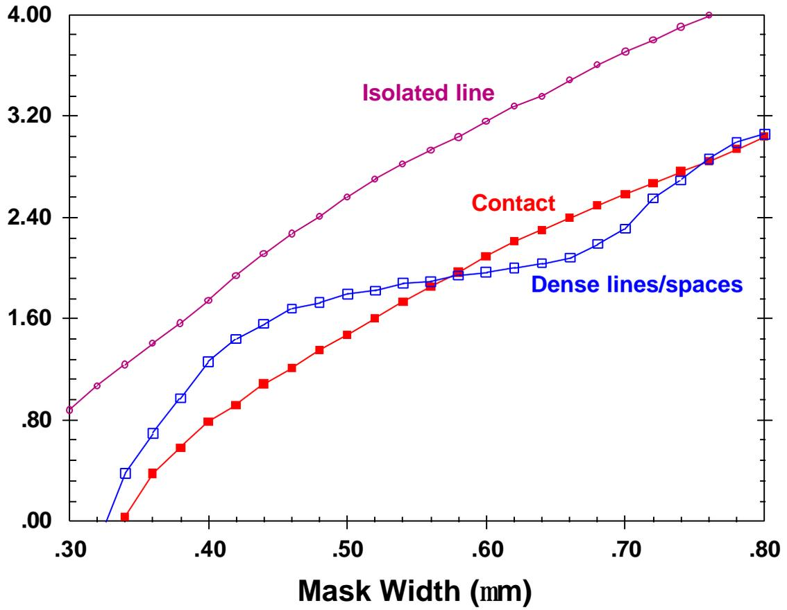
Figure 2. Comparison of the resolution for different feature types (i-line, NA = 0.54,  $\sigma = 0.5$ , typical resist on bare silicon).
