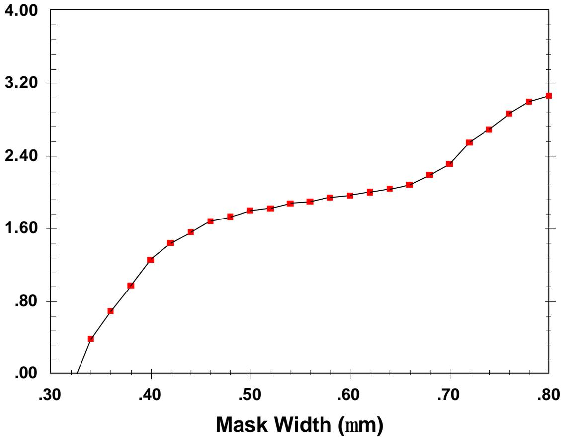
Figure 1. Resolution can be defined as the smallest feature which meets a given DOF specification. Shown are results for equal lines and spaces, i-line, NA = 0.54,  $\sigma = 0.5$ , typical resist on bare silicon.
