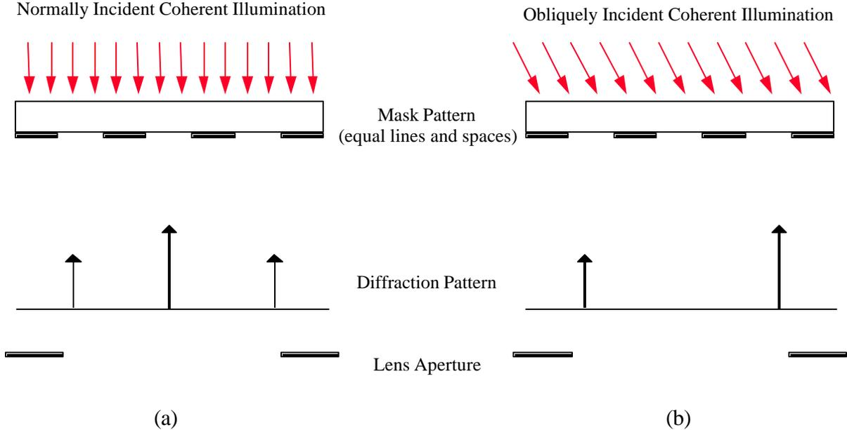
Figure 1. Resolution Limit for equal lines and spaces for (a) normally incident illumination and (b) oblique incidence.
