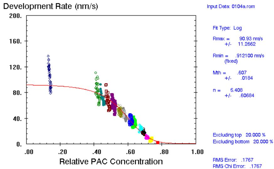
Figure 2: Plot showing the dissolution rate as a function of relative PAC concentration at 35°C developer temperature, 0.24425 N overlaid with the best fit to the original Mack development rate model.
