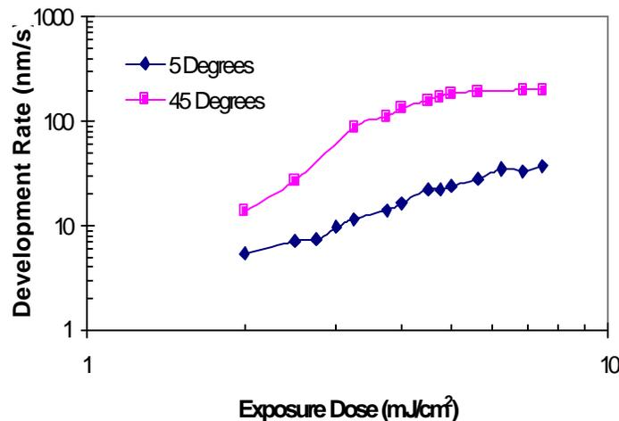
Figure 3: Development rate of APEX-E (averaged through the middle 20% of the resist thickness) as a function of exposure dose for different developer temperatures. At higher doses, higher developer temperature increases the dissolution rate. Higher developer temperature also increases the dissolution selectivity parameter  $n$ .
