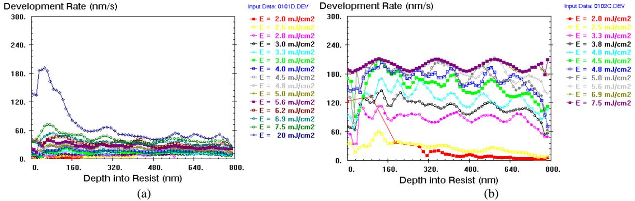
Figure 1: Dissolution rate data from the RDA-790 for APEX-E at developer temperatures (a) 5°C, and (b) 45°C.
