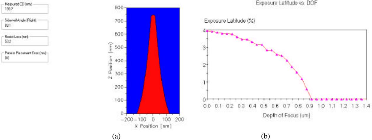
Figure 9. PROLITH simulated (a) resist profile for a binary 200nm line/space feature using MF-702 Developer at 20°C, and (b) Exposure Latitude vs. DOF analysis of a Focus-Exposure Matrix.
