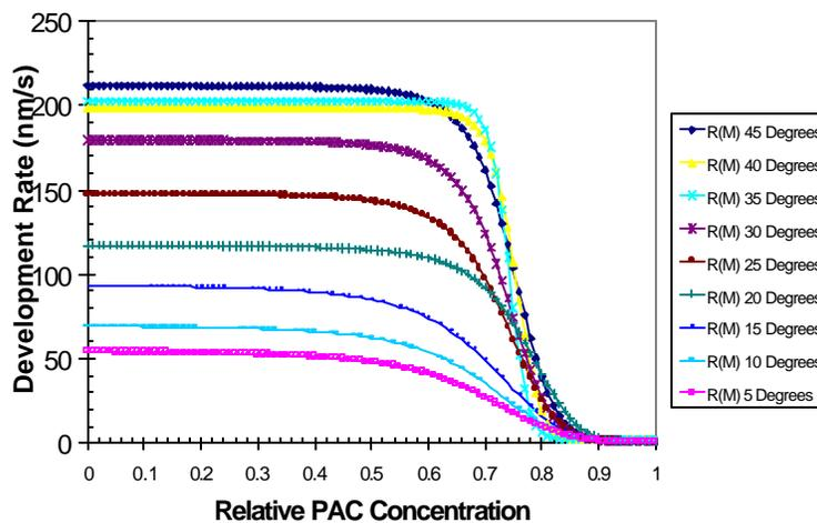
Figure 4: Comparison of the best-fit models of APEX-E for different developer temperatures shows the leveling off of develop rate at higher temperatures and exposure energies, the shift in  $m_{TH}$  and increasing dissolution selectivity parameter  $n$ .
