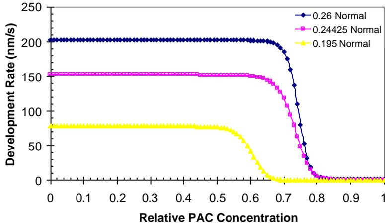
Figure 7: Comparison of the effect of developer normalities on the development rate of APEX-E at 35°C developer temperature. Shows the effects of decreasing maximum dissolution rate  $R_{max}$ , and shift in  $m_{TH}$
