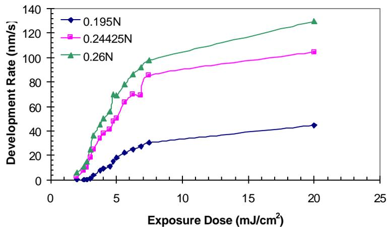
Figure 6: Development rate of APEX-E (averaged through the middle 20% of the resist thickness) as a function of exposure dose for different developer normalities at a developer temperature of 20°C. At all doses, lower developer normality decreases the dissolution rate, with higher doses receiving the greatest decrease. Lower developer normality also decreases the dissolution selectivity parameter  $n$ .
