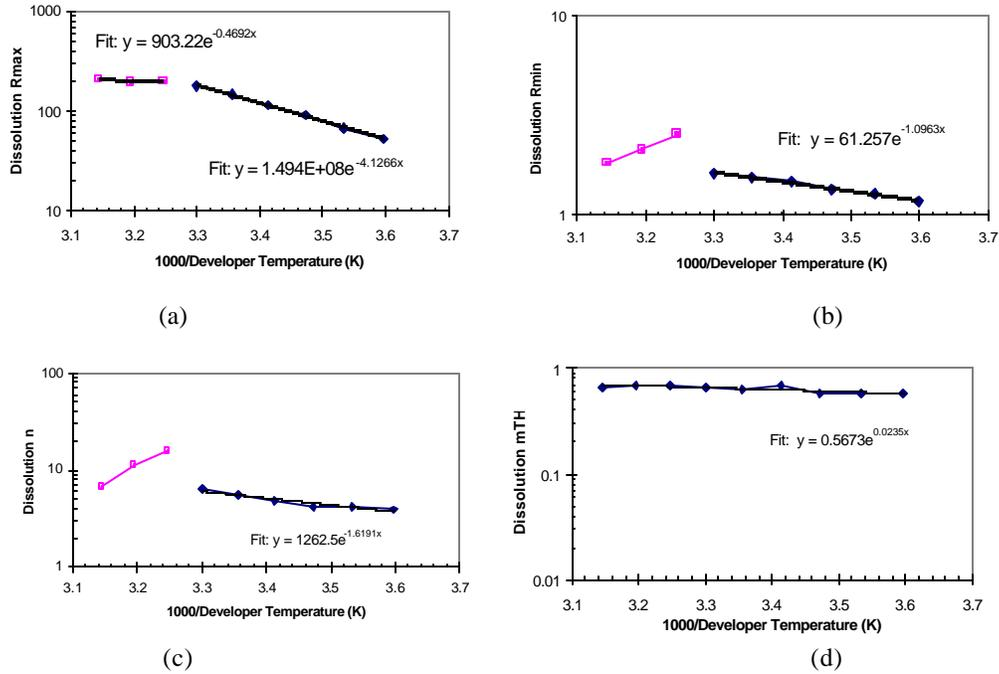
Figure 5. Arrhenius plots of (a) the maximum dissolution rate  $R_{max}$ , (b) the minimum dissolution rate  $R_{min}$ , (c) the dissolution selectivity parameter  $n$ , and (d) the threshold PAC concentration  $m_{TH}$ . Best fits to the Arrhenius equation are also shown.
