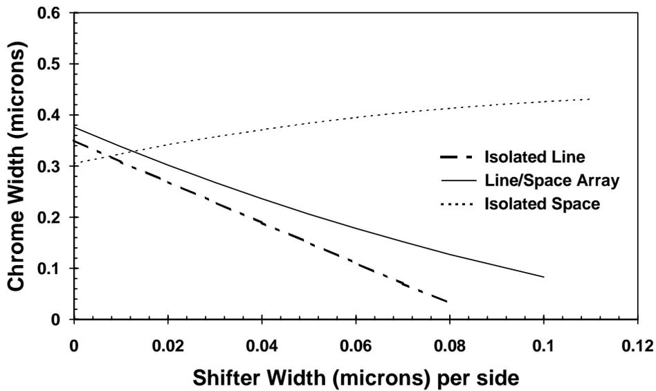
Figure 2: Design curves for rim shifted 0.35  $\mu\text{m}$  features (i-line,  $\text{NA} = 0.5$ ,  $\sigma = 0.4$ , SPR500 resist, bare Si wafer, 200  $\text{mJ}/\text{cm}^2$  exposure dose, simulated with PROLITH/2).
