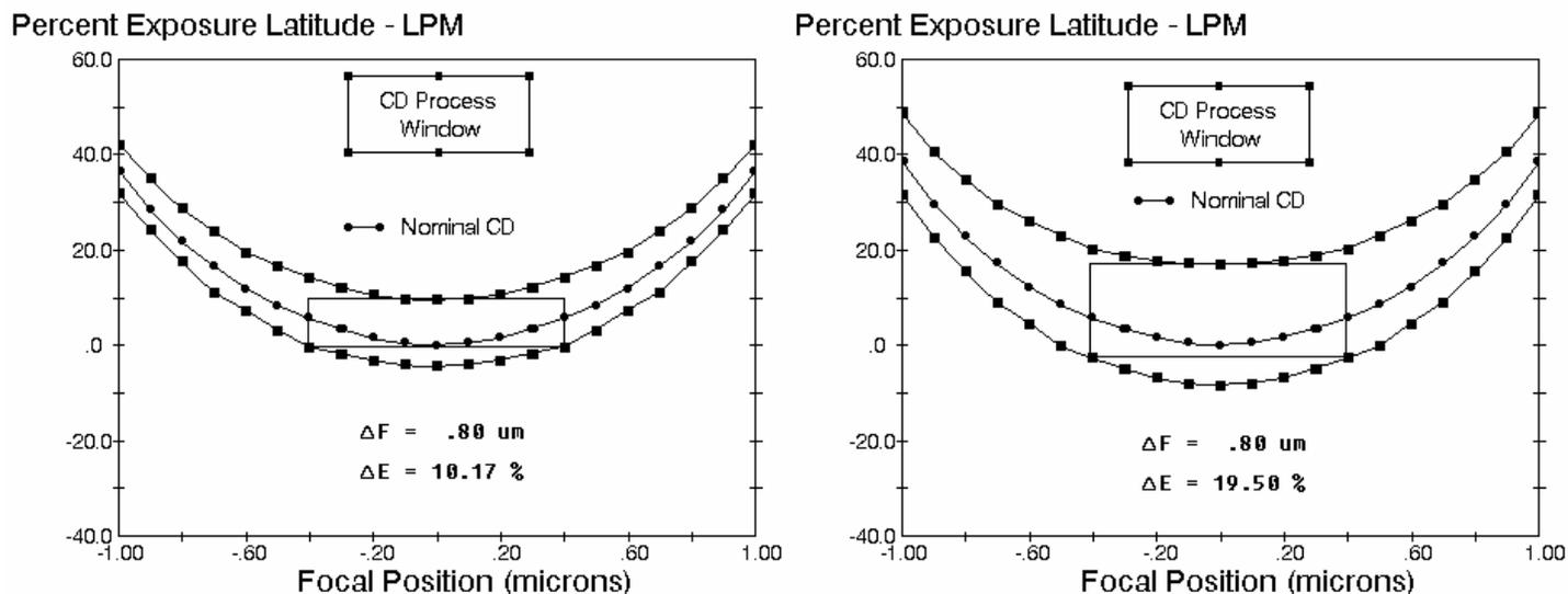
Figure 6. Comparison of process windows generated using the Lumped Parameter Model (LPM) for (a) no rim, and (b) a  $0.1 \mu\text{m}$  rim for a nominal  $0.4 \mu\text{m}$  isolated space (i-line,  $\text{NA} = 0.5$ ,  $\sigma = 0.4$ , simulated with PROLITH/2)
