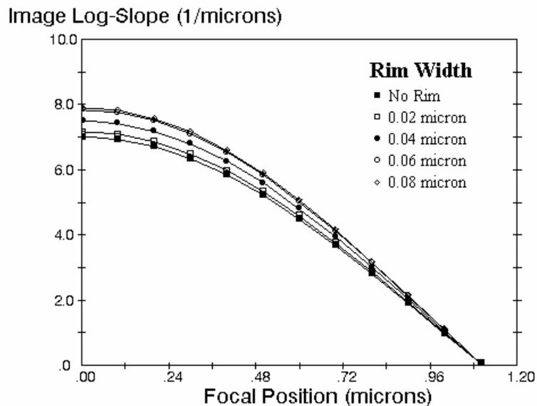
Figure 4. Log-slope defocus curves for a 0.35  $\mu\text{m}$  line/space array for varying amounts of rim shifter width (i-line, NA = 0.5,  $\sigma = 0.4$ , using chrome width as determined from the design curves of Figure 2, simulated with PROLITH/2).
