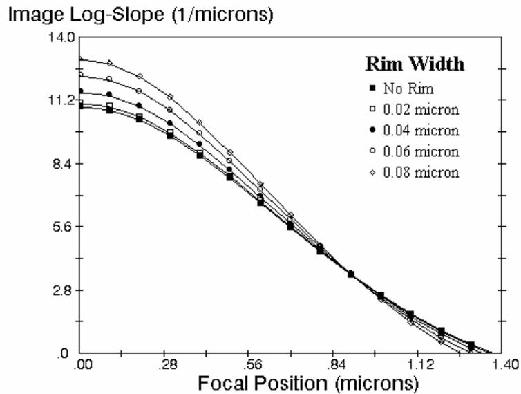
Figure 3. Log-slope defocus curves for a 0.35  $\mu\text{m}$  isolated line for varying amounts of rim shifter width (i-line, NA = 0.5,  $\sigma = 0.4$ , using chrome width as determined from the design curves of Figure 2, simulated with PROLITH/2).
