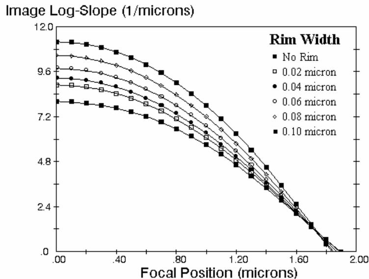
Figure 5. Log-slope defocus curves for a  $0.35 \mu\text{m}$  isolated space for varying amounts of rim shifter width (i-line,  $\text{NA} = 0.5$ ,  $\sigma = 0.4$ , using unshifted space widths as determined from the design curves of Figure 2, simulated with PROLITH/2).
