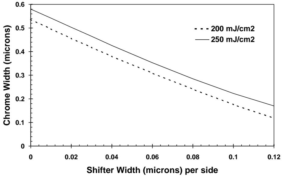
Figure 1: Design curves for a rim shifted 0.5  $\mu\text{m}$  isolated line for the two listed exposure doses (i-line,  $\text{NA} = 0.5$ ,  $\sigma = 0.4$ , SPR500 resist, bare Si wafer, simulated with PROLITH/2).
